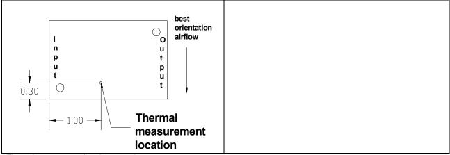
Thermal measurement location - top view
